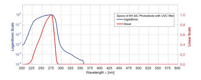
UVC-only SiC based UV photodiode A = 0,50 mm<sup>2</sup>
