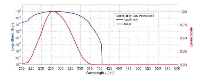
Broadband SiC based UV photodiode  $A = 1,82 \text{ mm}^2$
