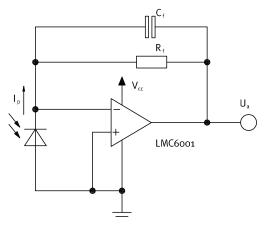
$U_a = I_p x R_f = o \dots \sim V_{cc}$
