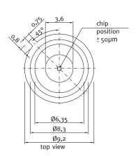
UVC-only SiC based UV photodiode A = 0,20 mm<sup>2</sup>
