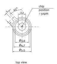
UVB-only SiC based UV photodiode A = 0,06 mm<sup>2</sup>
