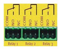
Three potential-free relays can be used for process control.
