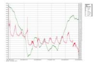
Using the software *Setup* the user customizes the properties of the UV Minilog. With the software *Reader* the USB data transfer ist started. The *Viewer* is used for graphical displaying. The data can be exported as a csv file for analyzing in standard software like Excel or Origin. The software *Online* is displaying online measurements.
